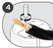
Push wires into disposer (do not displace cardboard shield) and replace electrical cover plate.
